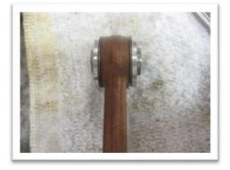
I use a West Bend 610 or 820 wrist pin, but either one needs to be machined to a 1.590 +/- .005 length to work in the AH-58 piston (see picture, below). I get the steel thrust washers from Engine Masters (Dave Bonbright).
