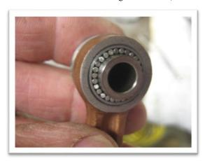
The West Bend wristpin has a thicker wall thickness so it is a little heavier. This seems to help bring the engine into a better balance. The West Bend wristpin is just a little more insurance in the reliability area. The pistons I have made use the West Bend circlips for the wristpin. Whichever circlip you use, always use new ones; it is cheap insurance.
