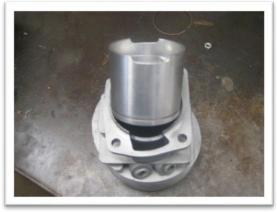
Next, I set the cylinder up for honing. I made a plate that mirrors the crankcase to hold the cylinder in a vice (see picture, next page). Pistons are hard to find for these engines, so I have had Billet pistons made by ARIAS in a .010 oversize to take a single 1mm ring (.039).
