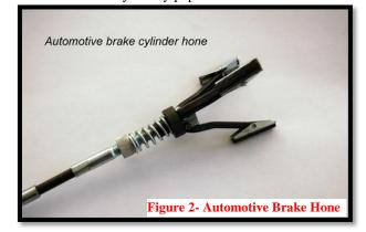
The brake cylinder hone leaves a surface that is too rough for the "O" rings the caliper and master cylinder pistons use. The simple solution I found to fix this is to wrap the hone stones with the sandpaper (Fig. 3) and repeat the process with the WD-40 as the lubricant. I wrap the paper around one stone and then around all three while I'm holding the stones together. Then I insert the hone and it will configure itself to the bore.
