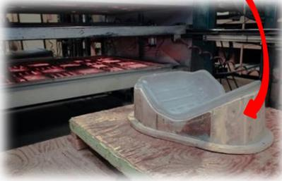
2. Lay a piece of heated polyethylene over the form.
