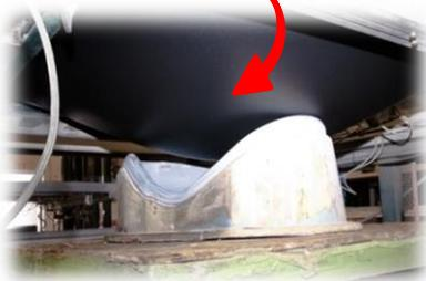
3. Apply suction to the form to pull the polyethylene tight to the form.
