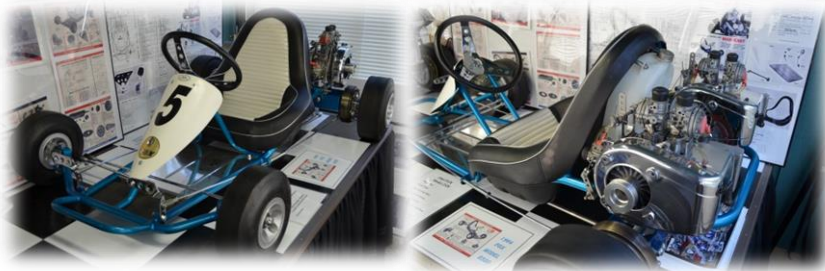
The 1964 Fox Box Mount was a revolutionary design that eliminated one bearing from the rear axle. This one has West Bends with triple, small throat carbs. The new frame design is very similar to the 1960 Sprint Kart.
