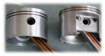
**Pistons** – Finding the right pistons was the biggest challenge because racing pistons for 820's are becoming nonexistent. The factory is looking at helping us out, but not in the near future. A friend of mine was able to purchase a stash of NOS Wiesco 9-port, thin-ring pistons and rings. He sent them to me and I'm building him four engines also. The piston on the left is a stock 820.
