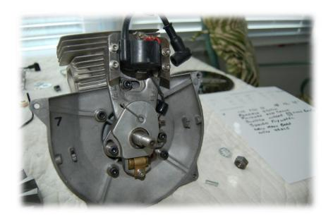
**Flywheel -** My sprint track racing engines have the flywheel fins cut down. Most of the engines I've purchased over the last few years had the fins removed back in the 60's. New Wico flywheels and stators that use points and condensers are becoming harder to find as the years grind on.
