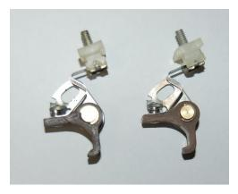
File the tip of the point assembly that contacts the crankshaft to a 45-degree angle until there's about a .030 (1/32) inch flat left.
