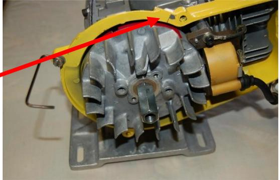
3. Assemble the coil in place - I use a .010 long piece of feeler stock to get the correct air gap between the flywheel magnets and the coil laminations.
