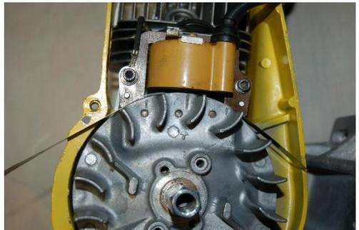
4. There is side play in the lamination slots. I usually push the coil to the left before tightening the screws.
