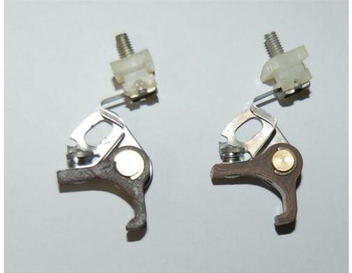
File the tip of the point assembly that contacts the crankshaft to a 45-degree angle until there's about a .030 (1/32) inch flat left.
