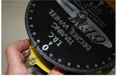
12. Rotate the engine to 20 degrees and put a small mark on the flywheel. Then move to 25 degrees and mark the flywheel. Continue to mark every 5 degrees to 40 degrees.
