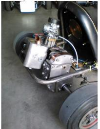
20 degrees. Mark the location and then remove engine and the mount from the gearbox.
