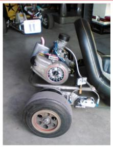
1.. Remove the gearbox mount from the engine and install the muffler without the gearbox.
