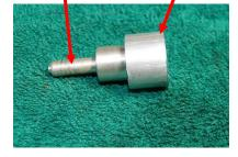
I found a .2493" diameter reamer at McMaster Carr, reamed the aluminum and the bushing pressed in with the gentle tap of a hammer. Now it was time to machine the carbs. I drilled the carbs
